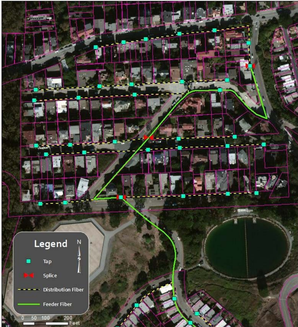
Figure 8: Sample FTTP Access Layer Design
