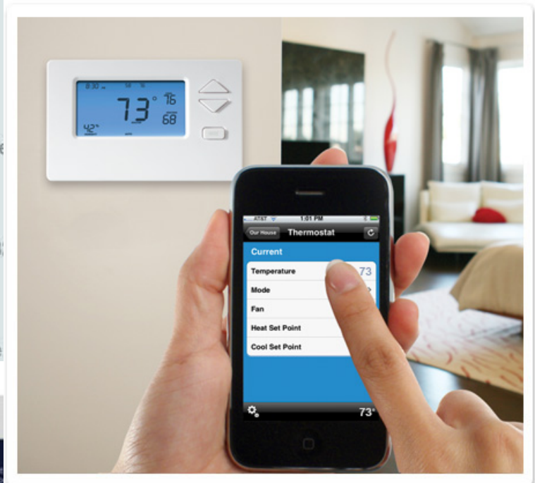
Pictured Above INSTEON Thermostat (#2441TH) controlled by an iPhone running INSTEON app. The app communicates to SmartLinc (#2412N) connected to a router and is accessible from home or anywhere in the world. Setup also requires Access Point (#2443).
