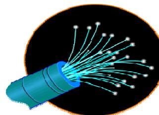
Fiber Optic Cables are thin strands of glass that carry light instead of electricity. Fiber optics are lighter, immune to electrical interference, and carry information faster than standard network cables.
