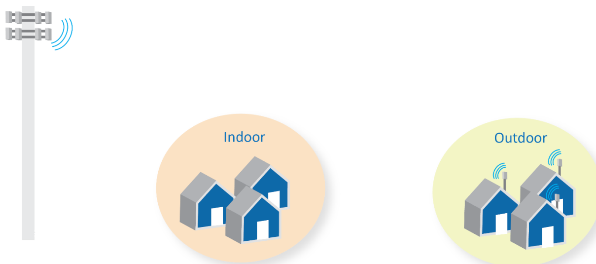
Figure 3: Sample Indoor and Outdoor Customer Antenna Configurations for a Fixed Wireless Network
