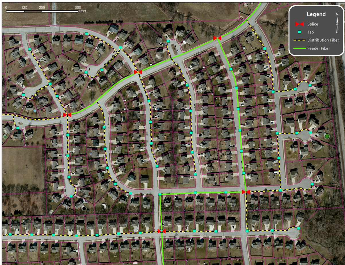
Figure 15: Sample FTTP Access Layer Design
