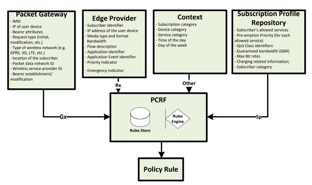
Figure 2: PCRF Analyzing Requests and Network Data and Provisioning a QoS Policy Rule
