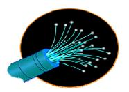
Fiber Optic Cables are thin strands of glass that carry light instead of electricity. Fiber optics are lighter, immune to electrical interference, and carry information faster than standard network cables.
